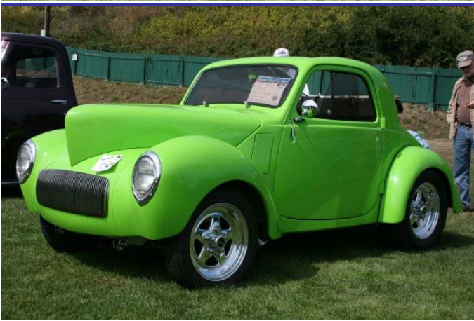
All Steel, hand-formed, ~3/4 scale Willis Front End— built by George McMurray, Sequim
